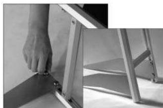
Screw and fasten the legs on the main body profile of the frame.
